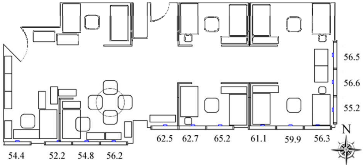
Figure 6 –Humidity Distribution – With an Open Window
