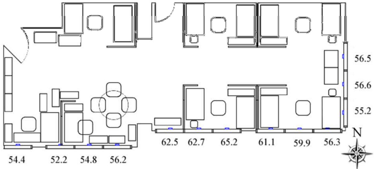
**Figure 6 –Humidity Distribution – With an Open Window**
