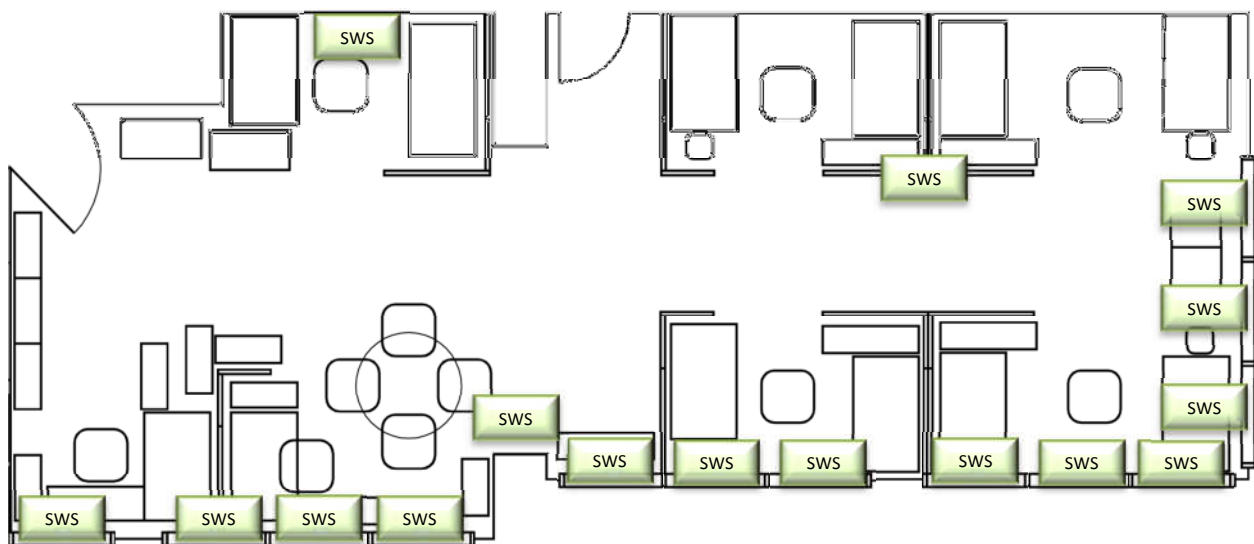
Figure 3 – Engineering Office Smart Window Sensors Locations
